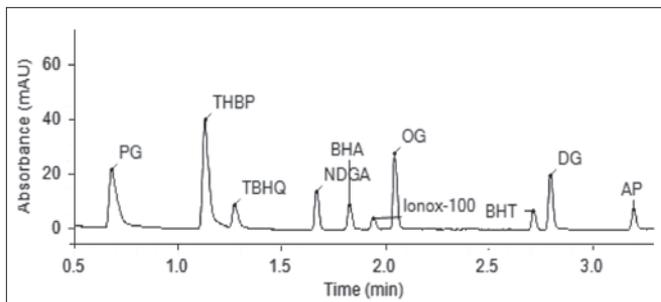
Figure 5. The chromatogram from the analysis standard solution of 10 antioxidants with a C18 UHPLC column.
