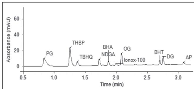
Figure 6. Chromatogram of the analysis of canola/olive oil spiked with 10 antioxidants with a C18 UHPLC column.
