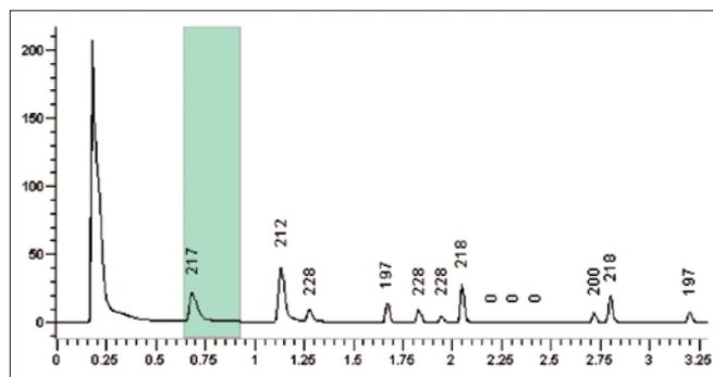
Figure 3. Chromatogram from the analysis of a standard with a C18 UHPLC column showing maximum wavelength absorbance for each peak.
