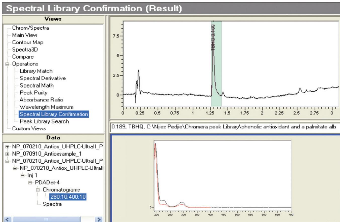
Figure 7. Chromatogram of the analysis of vegetable shortening and the spectra confirmation using a Chromera PDA spectral library.
