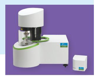
The GMD 8000 allows mixing of up to three gases, delivering a custom gas environment to the TGA 8000™ or other devices. The GMD 8000 has three gas inputs, each with its own mass flow controller (MFC). Gas mixing is customized via a Windows® PC-based software program. The customized mixed gas exits from a single outlet and is delivered to the sample through the TGA 8000 reactive gas line or a non-controlled input port of other devices.
