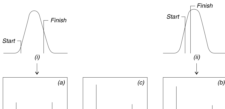
Figure 6 Slow scanning (i) of the mass spectrum over a GC peak for substance A produces a spectrum (a), but rapid scanning (ii) gives spectrum (b) which is much closer to the true spectrum (c)
