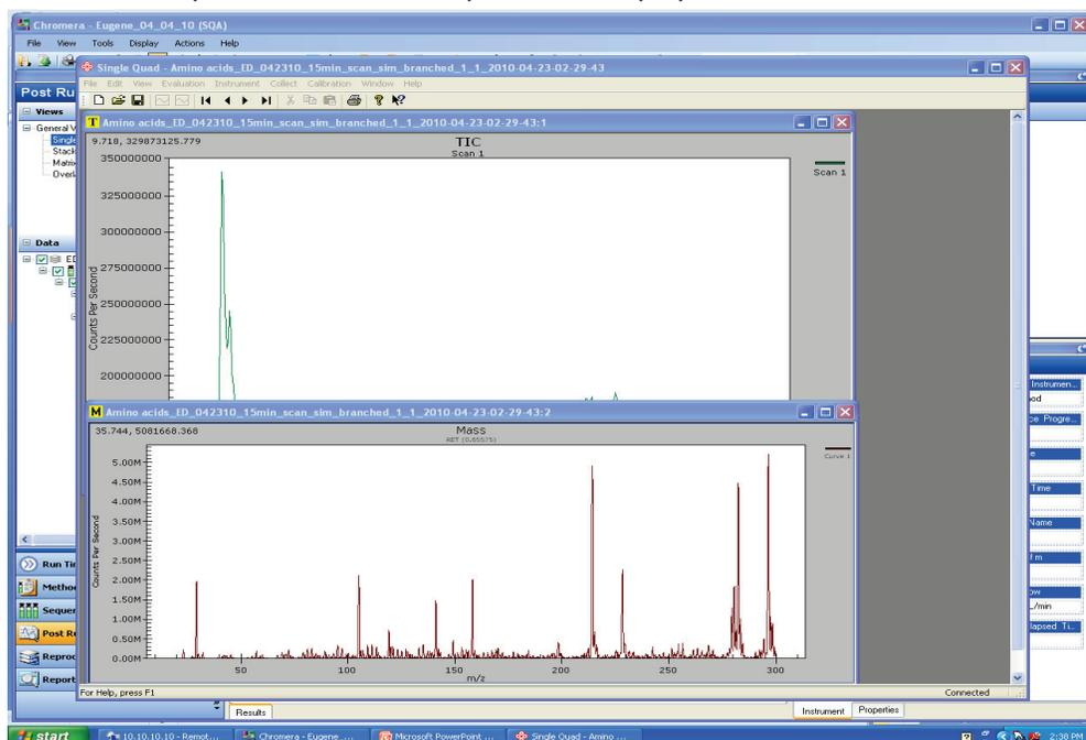
When a data file is opened a TIC window and a Mass spectrum window will be displayed.
