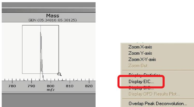
2. Release the button and select **Display EIC** from the menu. The **Extracted Ion Chromatogram** dialog displays.
