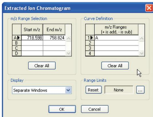
3. Click **OK** and the **EIC** is displayed. The EIC displays where in the chromatogram mass peaks occur with  $m/z$  values within the set  $m/z$  range.
