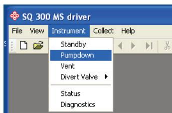
6. Open the **Status** screen by selecting **Status** from the **Instrument** menu to display vacuum status during pumpdown.
