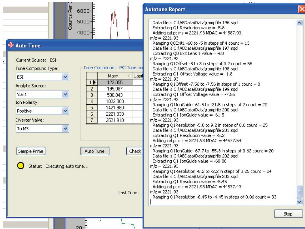
As Auto Tune runs in the positive ion mode, it creates the following three master tunes: **pos\_1k**, **pos\_5k**, and **pos\_10k** upon completion.
