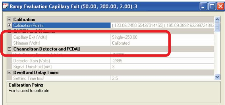
This indicates that to produce the maximum intensity  $m/z$  195 fragment ion, a **Capillary Exit** voltage of  $\sim$ 250 volts should be used.
