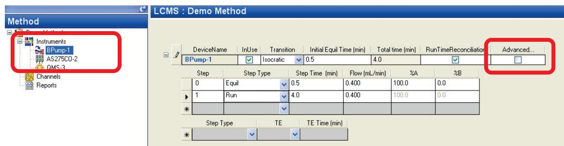
6. Click on **AS275CO-2** and enter the autosampler parameters. Click **Advanced** to show additional parameters.
