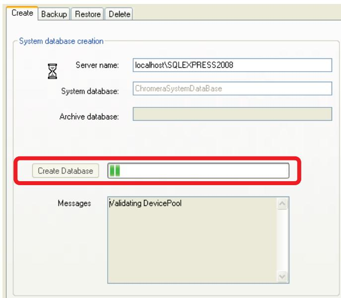
5. Upon successful completion, the next step is to configure "an instrument" for the system. In Chromera, an instrument is defined as a collection of devices. For example, individual **Devices** such as Flexar or Series 200 autosamplers, pumps and detectors are combined to create an instrument. In addition, a **Port Name** (for communication to each device) must also be defined in the Instrument configuration. Next create an **LCMS** instrument to use with the SQ 300 MS in a system.
