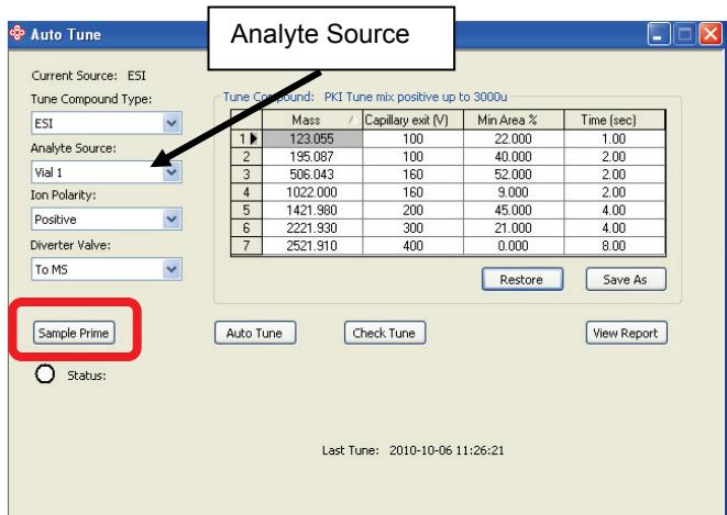
7. Click on the **Sample Prime** button and the **Tune Setup** dialog displays.
