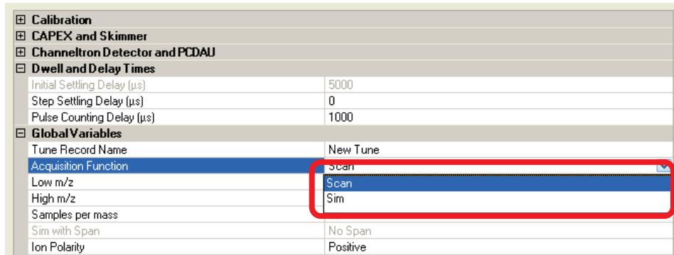
12. To set the specific SIM mass, select **Low m/z**, type your value, and press **Enter**. This example uses **m/z 609.3**.
