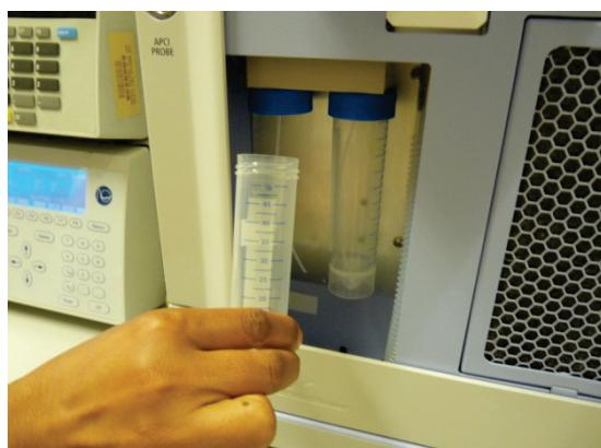
The calibration vial removed
