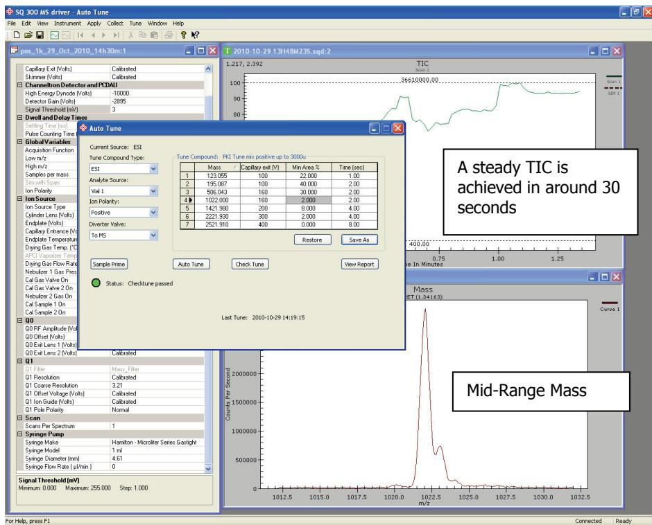
10. While viewing the **Mid-Range Mass**, you can adjust the source position by turning the indicated controls for maximum sensitivity.
