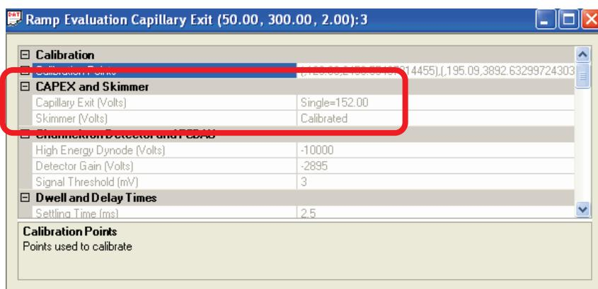
With a typical "bell shaped curve" as is demonstrated here, any value near the maximum will be perfectly acceptable. So in this example, any value in between 150 to 160 volts will provide the maximum signal intensity for reserpine.
