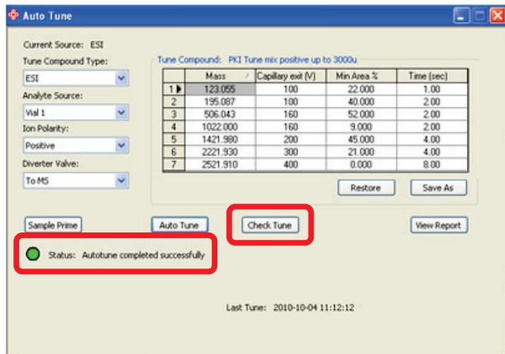
12. After auto tune is complete, click on **Check Tune**. The **Status** light will turn **yellow** and **Status: Executing check tune** displays. If a significant amount of time passes between the completion of Auto Tune and the execution of Check Tune, click the "Sample Prime" button to get the calibration mixture flowing again.
