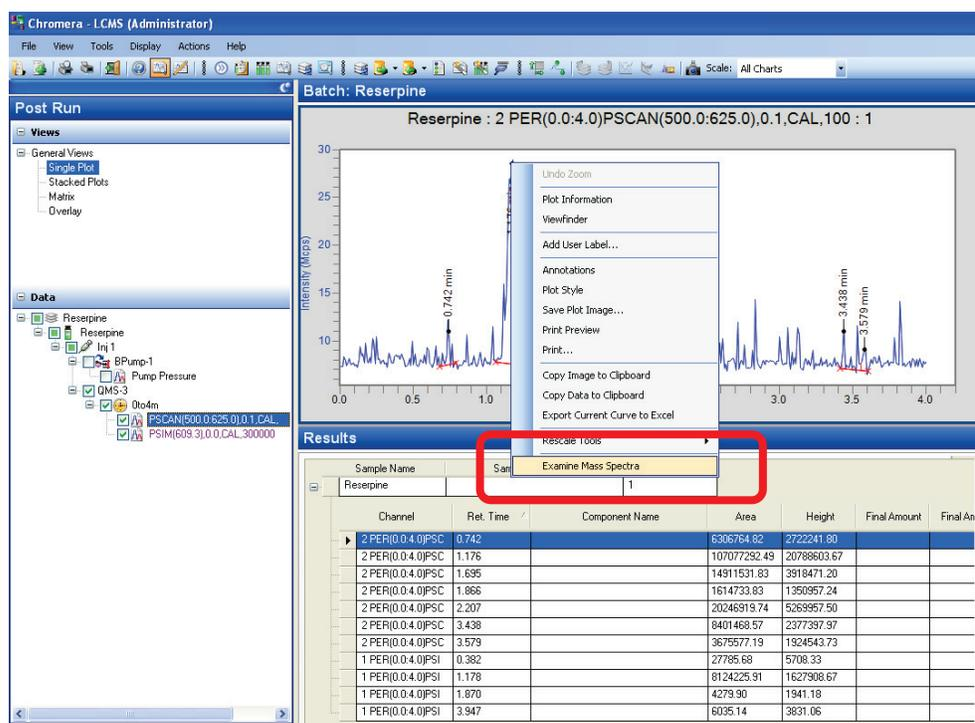
Another way to enter the mass spectral processing domain (demonstrated on a different data file) is to select **Examine Spectra** from the Chromera **Actions** menu.
