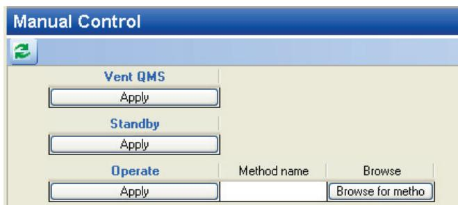
5. To verify the methods work with Chromera, in the **Standby** row click **Apply**. Observe that in the **Status Panel**, the **MS Detector State** displays **Standby**.
