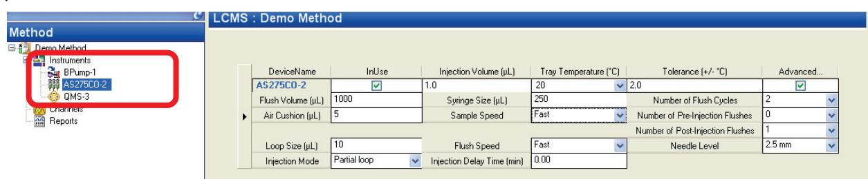
7. Click on **QMS-3** in order to link the MS Method previously defined in the SQ MS driver software to the Chromera method being defined.
