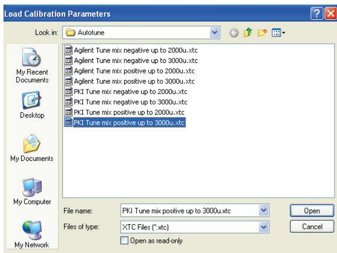
5. For Positive ion, highlight **PKI tune mix positive up to 3000u** and simply double-click on it. If calibration is only required up to 2000u, then the **PKI tune mix positive up to 2000u** file is available to use.
