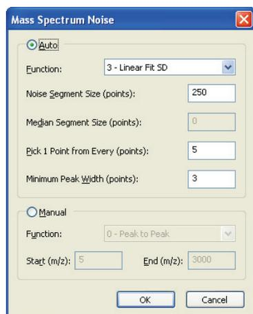
2. To detect the noise manually, select **Manual** and enter a mass range where there are not any peaks.
