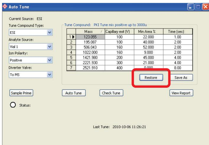
4. In the **Auto Tune** dialog, select a tuning compound reference file by clicking on **Restore**. This displays the **Load Calibration Parameters** screen.
