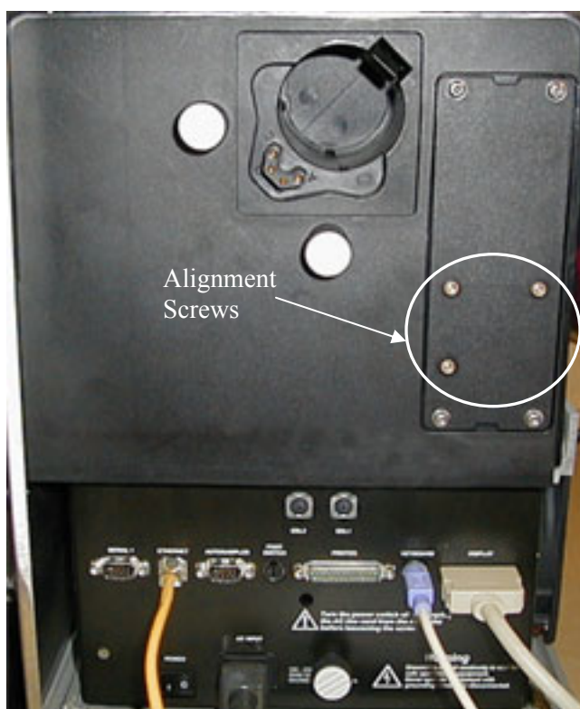
Figure 9- 19 Location of the alignment screws of the deuterium lamp.
