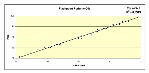
Fig. 1: MINIFLASH vs. automated Pensky Martens, performed by Henkel Germany. PMA methods: ISO 2719, EN 22719, ASTM D93.
