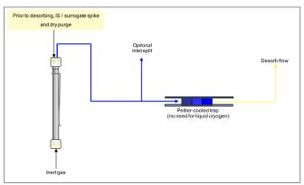
*Figure 1.* Sample tube desorption.
