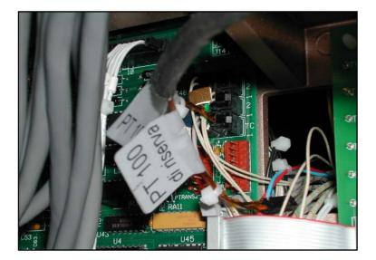
Step 7- Connect transfer line power supply (220 V only) to distribution board TB1 – AUX AC (position 1) and the return to an available MACC connection (position 4 or 5). Ground has to be connected to GC chassis ground.
