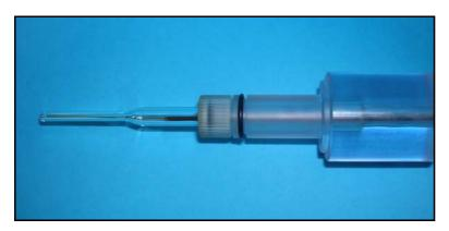
This figure shows the transfer line already connected to ICP-MS and ready to be used.
