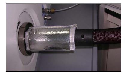
Column guard tube is only intended to protect the column end and the transfer line end when ICPMS injector is removed and transfer line is not in place.
