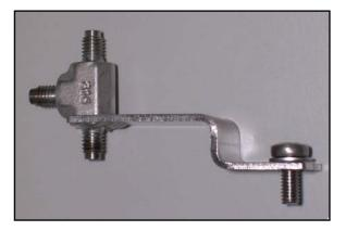
**d)** two deactivated silica column terminals (one 0.25 mm x 150 cm; one 0.32 mm x 150 cm to cut on appropriate lenght), with glass column connector and 1/16" female with ferrule
