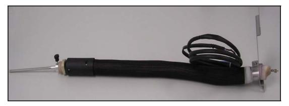
b) Dummy injector (make up gas preheat) 300 °C max operating temperature
