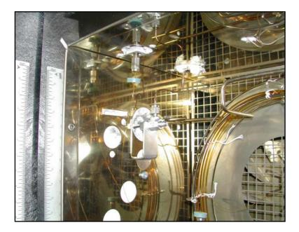
A 1/16" nut with a graphite/vespel or graphite ferula is used to tight the deactivate column to the desired length inside the transfer line.
