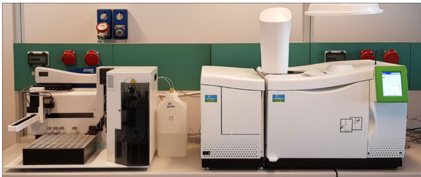
Figure 1. System P&T with Clarus SQ 8 GC/MS.
