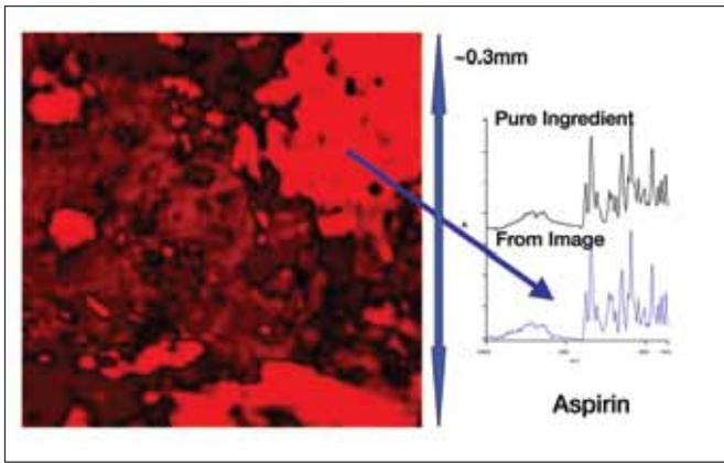
Figure 8a. Analgesic tablet – coarse structure – aspirin.
