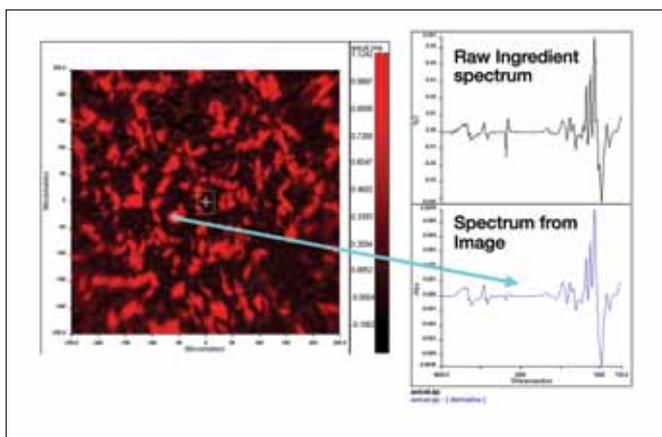
Figure 5a. Least squares fitted image for microcrystalline cellulose.
