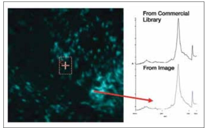
Figure 8d. Revealing minor constituents – calcium carbonate.
