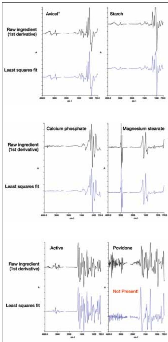
Figure 4. Testing for presence of raw ingredients.
