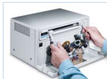
Figure 6. Easy interchange of FIMS absorption cell.
