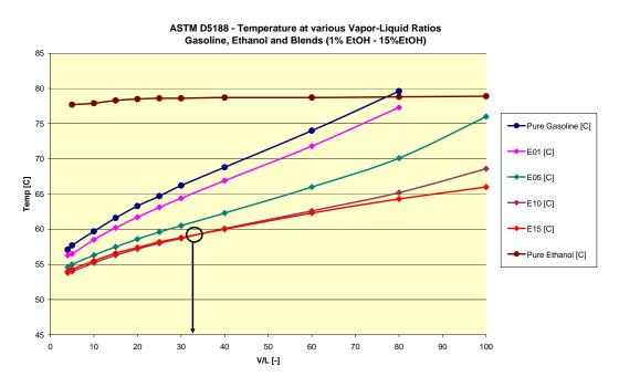
Fig 1: Temperature changes at various V/L ratio for 1%, 5%, 10% and 15% Gasoline-Ethanol blends. Highlighted is  $T_{(V/L)} = \sim 35$ .
