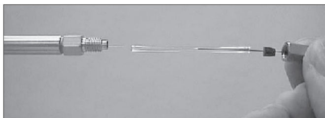
Figure 8. Hourglass guides restrictor into capillary column.
