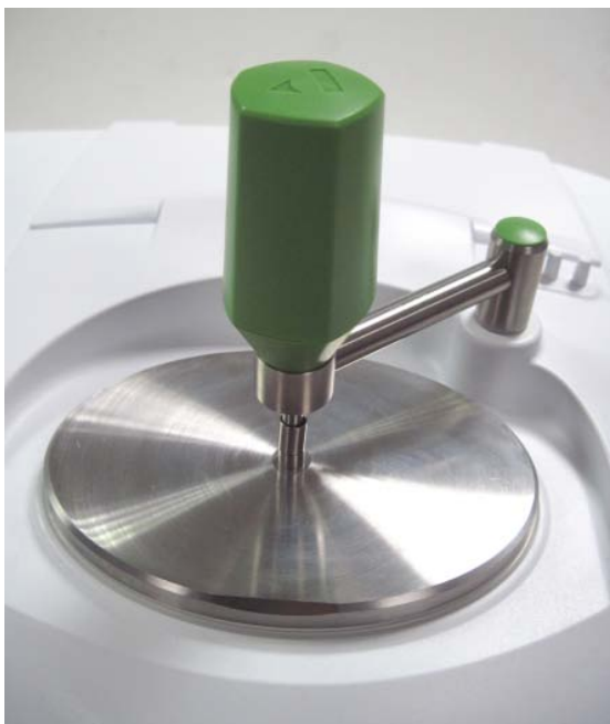
Figure 11 Using the pressure arm and medium shoe to cover the volatiles cup
