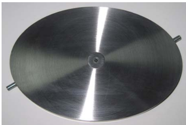
Figure 13 Fixing screws captured in top-plate
