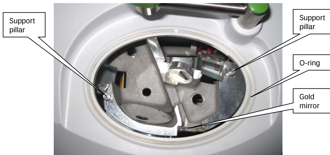
Figure 14 UATR with top-plate removed
