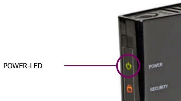
**Abb. 19. POWER-LED am Wireless Router**
