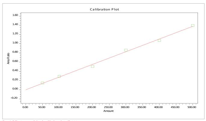
${\it Figure~2.}~ Calibration~ curve~ of~ ethanol~ used~ for~ the~ analysis~ of~ fruit~ juice.$
