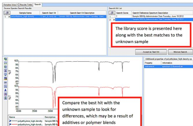
Figure 5. Example output from the "ScanAlyze" analysis.
