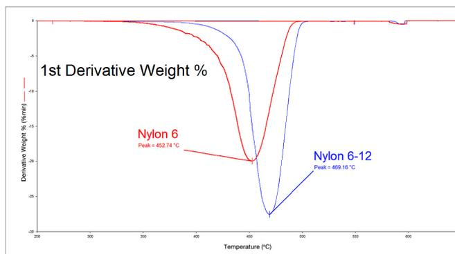
Figure 11. Example usage of the 1<sup>st</sup> derivative plots to determine identity of a polymer. In this case, there is a clear difference between the two forms of nylon.
