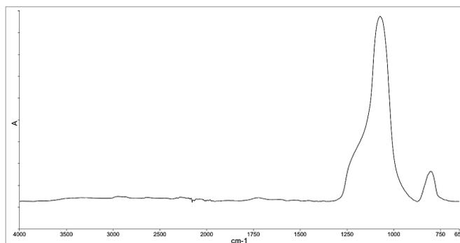
Figure 12. FT-IR analysis of the ash remaining in a TGA pan.
