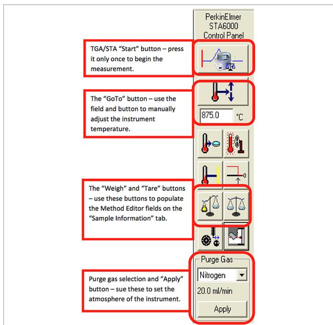
Figure 9. TGA/STA control panel.
