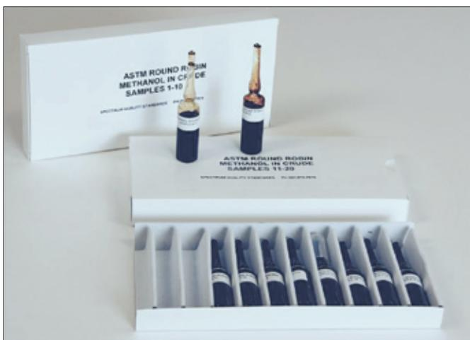
Figure 8. ASTM® D7059 round-robin validation samples.
