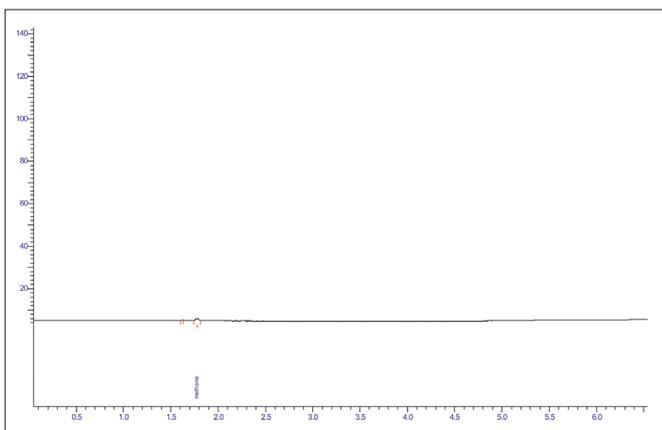
Figure 2. Chromatogram of blank (15 mL water).
