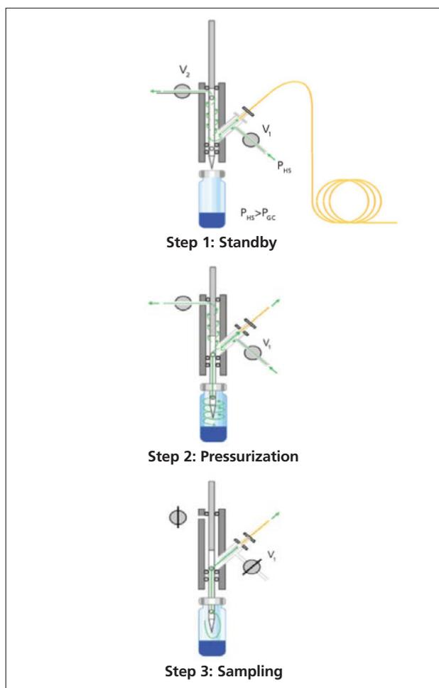
Figure 2. Pressure-balanced process.
