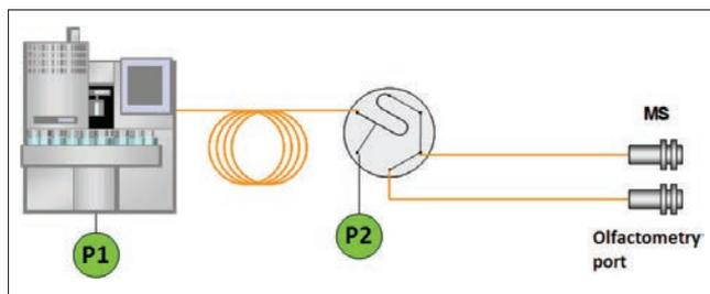
Figure 1. Schematic of the separation. For wet needle analysis the headspace system was removed and the capillary injector was used instead.
