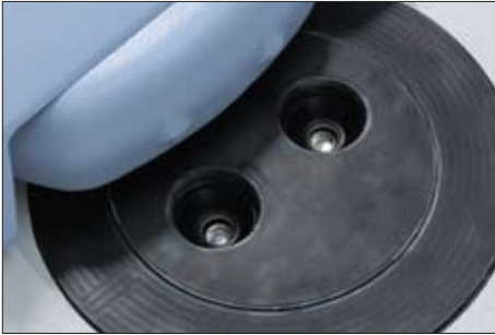
Figure 1. Double-furnace design allows the direct measurement of heat flow.
