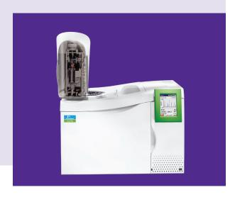
The PerkinElmer Clarus® 590 Gas Chromatograph (GC) is a fully automated gas chromatograph. The system offers the capabilities required for laboratories performing large numbers of routine analyses as well as those involved in research and development. All instrument functions are set up and monitored through a touch screen. The intuitive graphical user interface includes a real-time chromatogram display and eight-language support.
