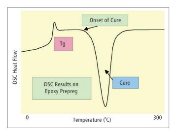
The DSC results, obtained at a heating rate of 20 °C/min, show that the Tg or softening of the epoxy prepreg material occurs at 60 °C. With further heating, the epoxy resin undergoes cure and crosslinking and this is observed as a large exothermic peak with a peak temperature of 160 °C. The peak temperature is equivalent to the point at which the resin achieves its maximum rate of cure.
