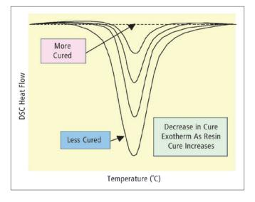
For electronic materials, the cure associated with an epoxy thermosetting resin may follow two distinctly different reaction mechanisms:
