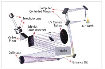
Figure 1. Avio 500 ICP-OES optical diagram.
