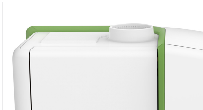
Figure 1. Vent for the Avio 200 ICP torch.
