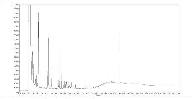
Figure 2. Chromatogram of Gasoline and Motor oil, run under the conditions in Table 1.
