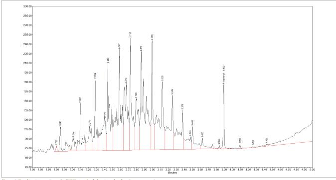
Figure 4. Baseline integration of a DRO standard showing the diesel range organics.
