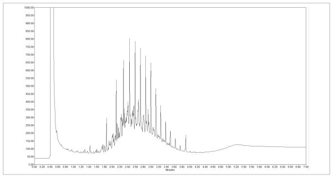
*Figure 1.* Chromatogram of Diesel fuel standard run under the conditions listed in Table 1.
