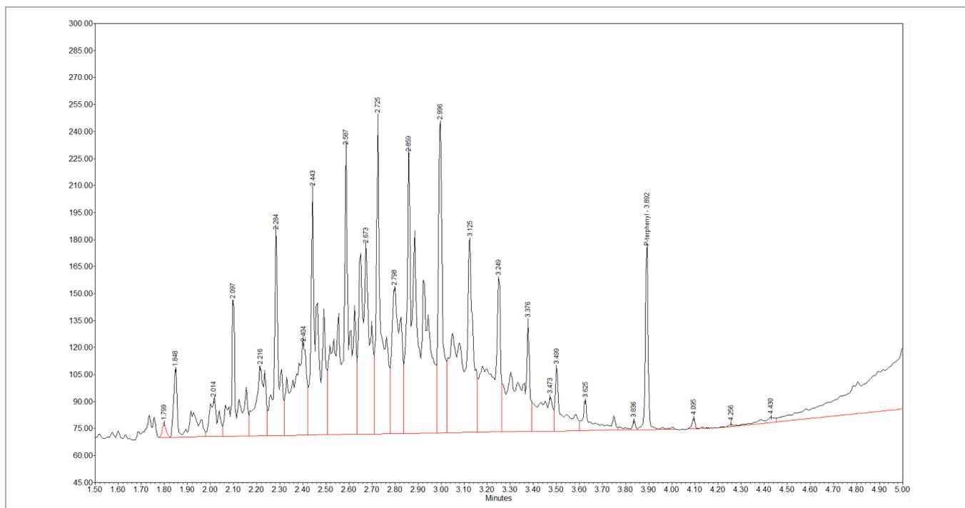
Figure 4. Baseline integration of a DRO standard showing the diesel range organics.
