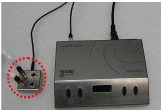
Figure 40 Connecting the two stirrer control cables
