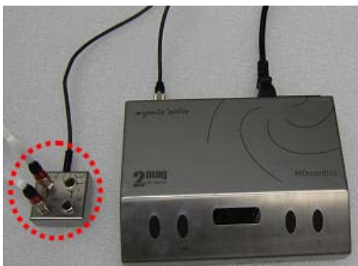
Figure 52 Connecting two stirrer control cables
