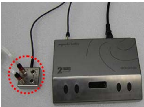
Figure 8 Connecting two stirrer control cables
