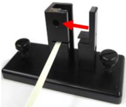
Figure 43 Assembling the single cell holder
