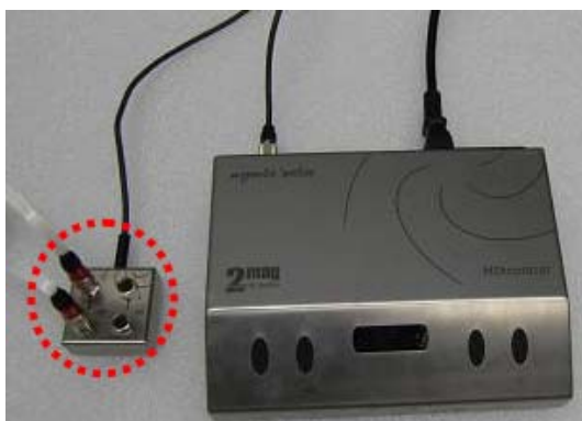
Figure 46 Connecting the two stirrer control cables
