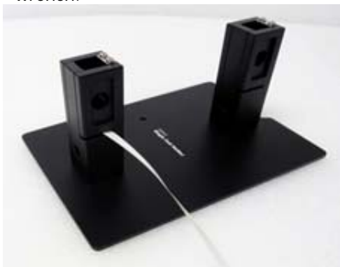
Figure 20 Assembling the single cell holder
