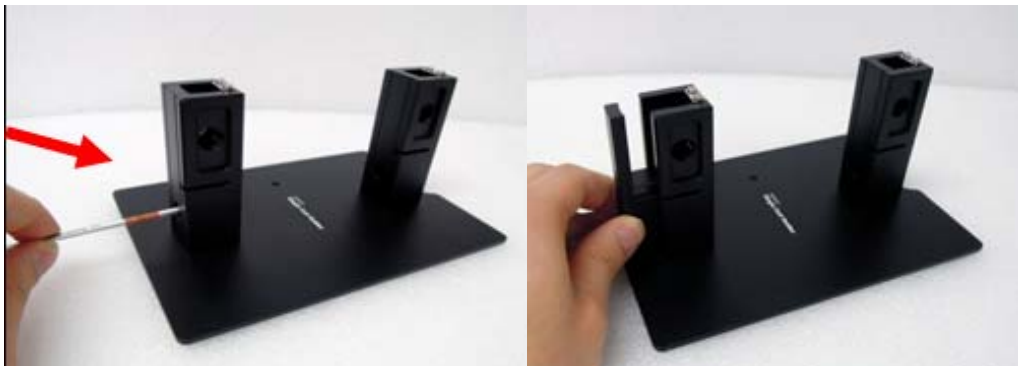
Figure 18 Removing the screw in the single cell holder
