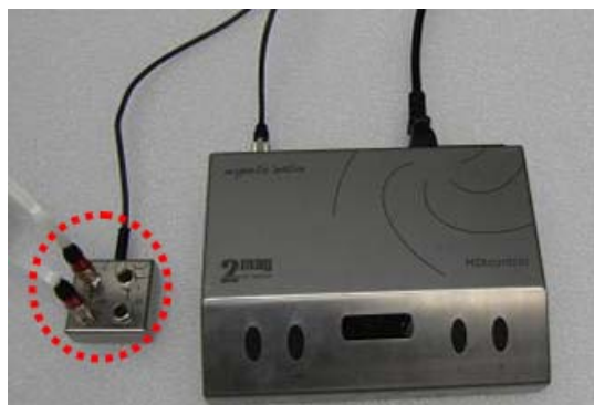
Figure 17 Connecting the two stirrer control cables
