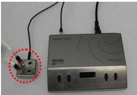
Figure 30 Connecting two stirrer control cables
