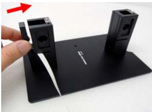
Figure 19 Inserting the stirrer head
