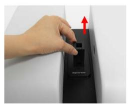
Figure 4 Removing the existing cell holder
