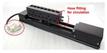
Figure 3 Lambda 265 Water Jacketed 8-position Multi-Cell Holder
