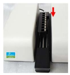
Figure 5 Water Jacketed 8-Position Multi-Cell Holder (or 8-Position Multi-Cell Holder)
