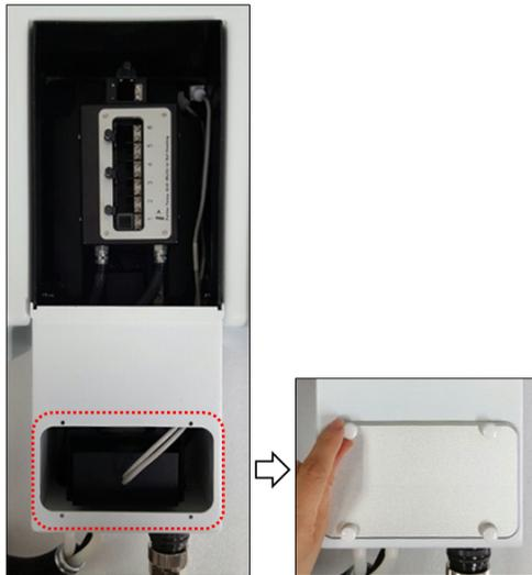
**Figure 17 Stuffing the probe line into the cell compartment**
