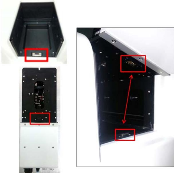
**Figure 11. Connecting the communication ports**
