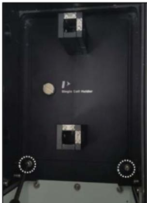
**Figure 8 Location of Phillips round head screws with washer**
