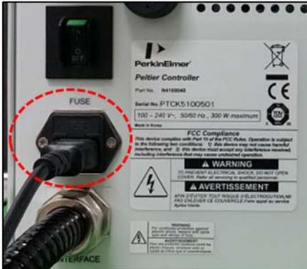
Figure 19 Connecting the power cord
