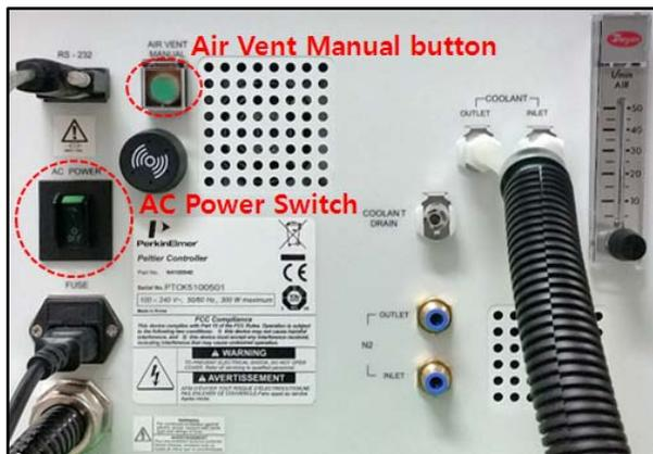
Figure 20 Turn on the AC power switch
