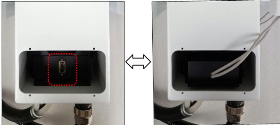
**Figure 16 Connecting the temperature probe**
