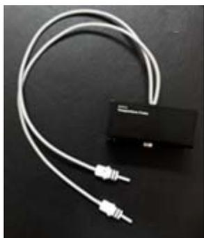
**Figure 4 Temperature probe**
