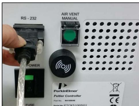
**Figure 18 Connecting the Peltier Controller with the PC**
