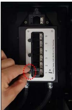
**Figure 24 Pull out the cell**
