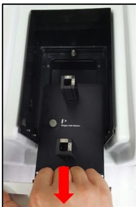
**Figure 9 Pulling out the cell holder and base plate**
