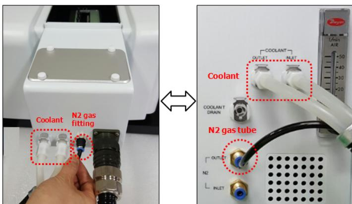
**Figure 14** Connecting the coolant inlet/outlet and N<sub>2</sub> gas fitting
