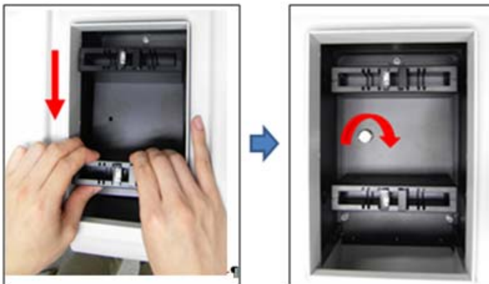
Figure 6 Inserting the variable pathlength cuvette holder
