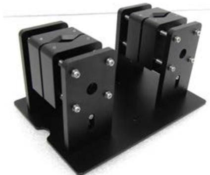
**Figure 1** Lambda 365 Test Tube Holder [P/N: N4101018]
