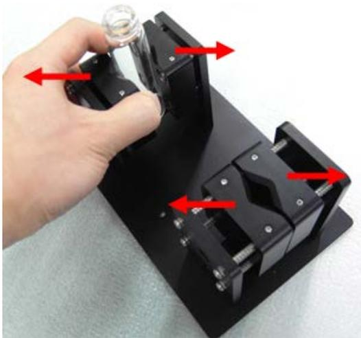
**Figure 9** Inserting the test tube
