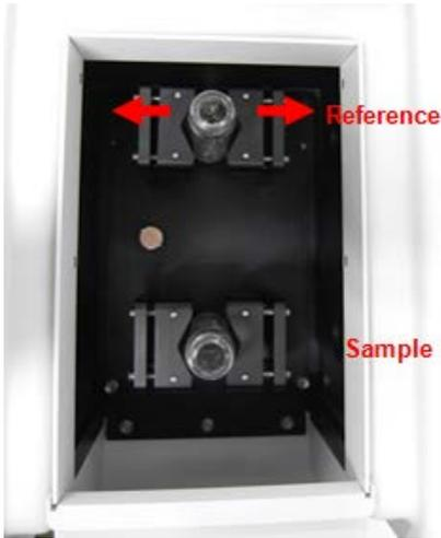
**Figure 8** Inserting the test tube holder
