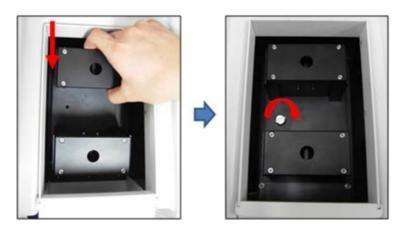
Figure 8 Inserting the Fixed Angle Reflectance Holder
