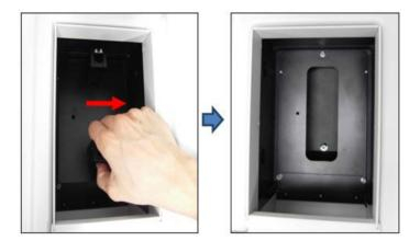
Figure 7 Pulling out the cell holder
