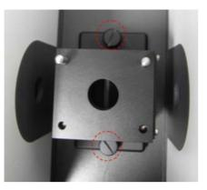
Figure 5 Installing the reflectance holder
