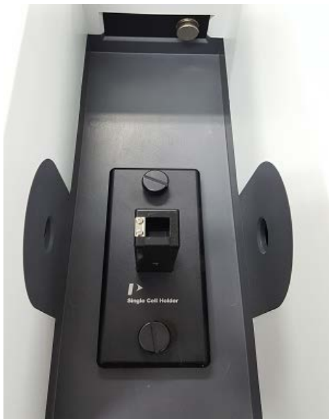
Figure 10 Taking apart the existing cell holder
