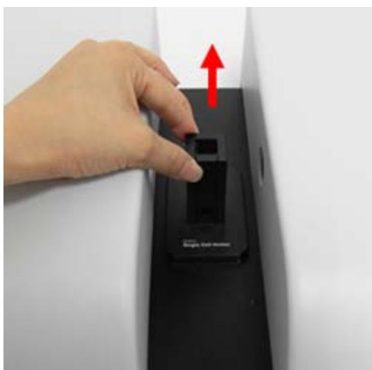
Figure 4 Removing the existing cell holder
