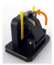
Figure 6 Closing the fixing arm on the sample
