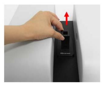
Figure 3 Removing the existing cell holder
