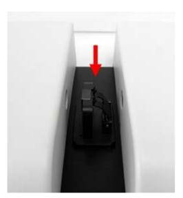
Figure 4 Install the Advanced Transmission Holder
