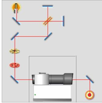
Figure 4. Spectrum 10 instrument beampath with HTM.
